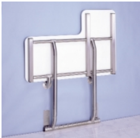
U934-1-Surface Mounted Retractable Shower Seat. Seat is fabricated of 2½" thick foam rubber cushion covered in white naugahyde. Entire frame is fabricated of type 304 #18 gauge stainless steel with a #4 satin finish. Uni-leg design allows easy transfer from wheel chair to seat from any direction. Overall Size: 18½"W x 15"D
