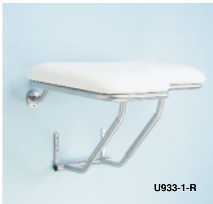
U933-1-Surface Mounted Retractable Shower Seat. Seat frame and supports are fabricated of 1¼" O.D. #18 gauge stainless steel tubing with a #4 satin finish. Seat cushion is constructed of 2½" thick foam rubber and covered in white naugahyde. Overall Size: 32"W x 20"D Specify right (R) or left (L) hand seat.
