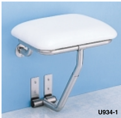
U934-1-Surface Mounted Retractable Shower Seat. Seat is fabricated of 2½" thick foam rubber cushion covered in white naugahyde. Entire frame is fabricated of type 304 #18 gauge stainless steel with a #4 satin finish. Uni-leg design allows easy transfer from wheel chair to seat from any direction. Overall Size: 18½"W x 15"D
